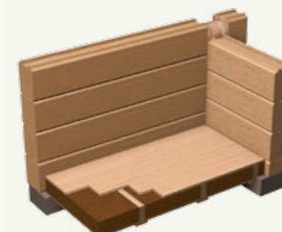
Massive log wall
